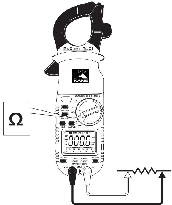
• **A** Do not measure resistance on a live circuit.
